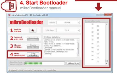
Start bootloader by clicking on the **Begin uploading** button. Click on the **Show Activity** button to view the operation of the bootloader.
